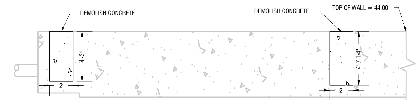
SCREENING DEMOLITION PROFILE VIEW SECTION A-A' NTS
